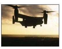
hover, and vertical landing qualities of a helicopter with the long-range, fuel efficiency, and speed characteristics of a turboprop aircraft.
